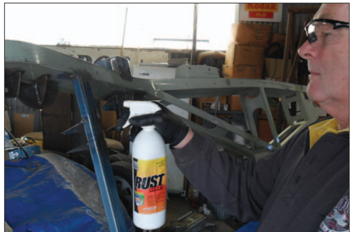
ABOVE: Next all of the surface rusted areas were treated with RustBlast to bring them back to shiny bare metal ready for painting. Spray it on, keep damp for 10 minutes and then wash it off.
