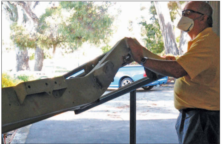
ABOVE: The etch primed areas of the chassis were given a scuff-down with dry 240 sand paper to give it a smoother surface, but still with some 'key' that would allow the RustSeal paint to adhere to it properly.
