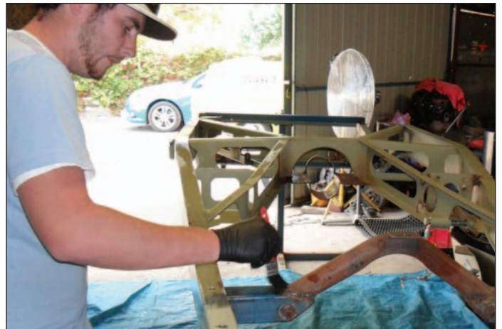
ABOVE: AquaKlean was used to clean any evidence of oiliness or grease from the surface of the chassis. This is simply painted on with a cheap brush and washed off with clear water.
