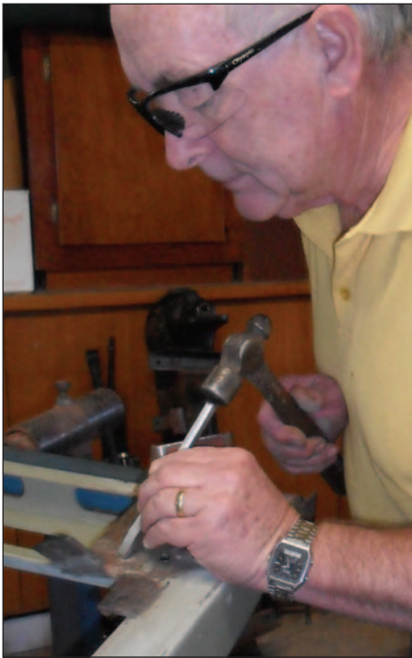
ABOVE: A small cold chisel was used to remove odd spots of weld spatter from around all of the brackets and crossmembers so that they wouldn't show up after painting.
