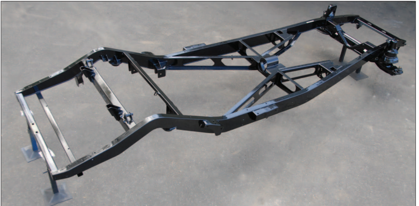
ABOVE: Finally a finished, painted chassis. The BlackTop finish coats came up superbly glossy and smooth right off the spray gun. No further finishing will be required, just paint all of the suspension pieces the same and start bolting it all back together.
